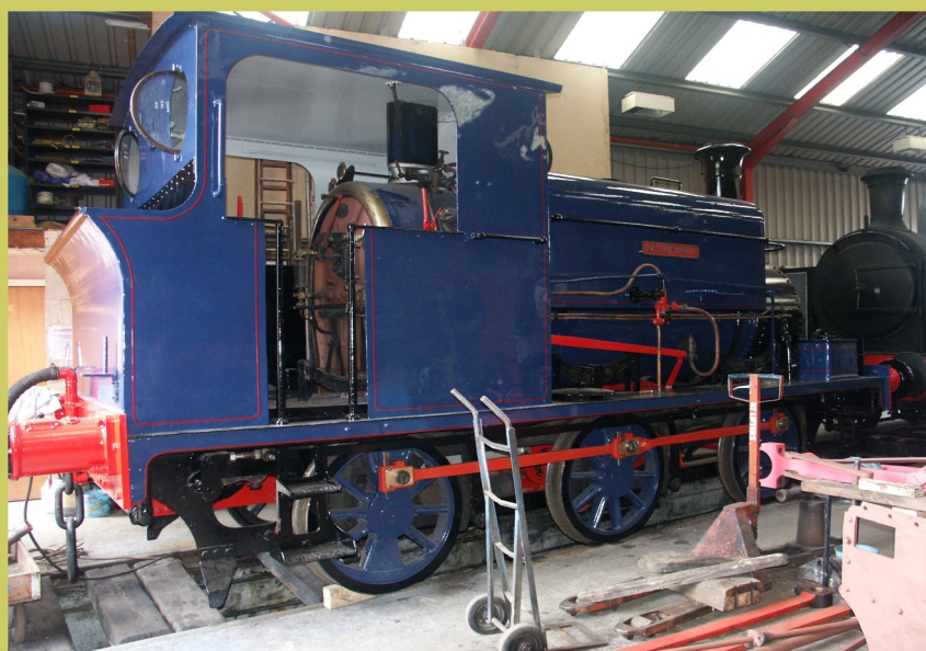
Manning Wardle 0-6-0 ST 1601/1903 Matthew Murray reaches its final stages of rebuild revealing the newly applied final coat of Longmoor Railway style blue with red lining, 8 May 2010 (Andrew Johnson)
