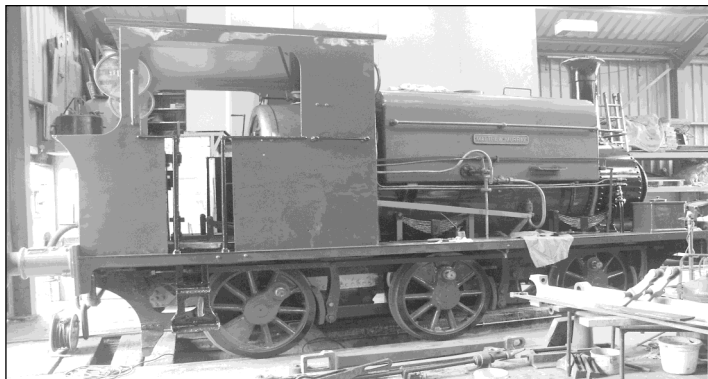
Manning Wardle 0-6-0ST Matthew Murray mas- querading as a 2-2-2ST, seen in the workshops on 10 April 2010 prior to final painting and lining out and fitting of con- nection rods
