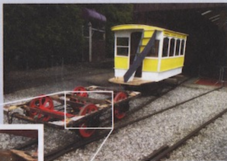
Detail showing the different profile of tram wheels, compared to the more familiar train wheels.
