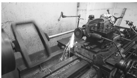
Brookes valve rod being ground
