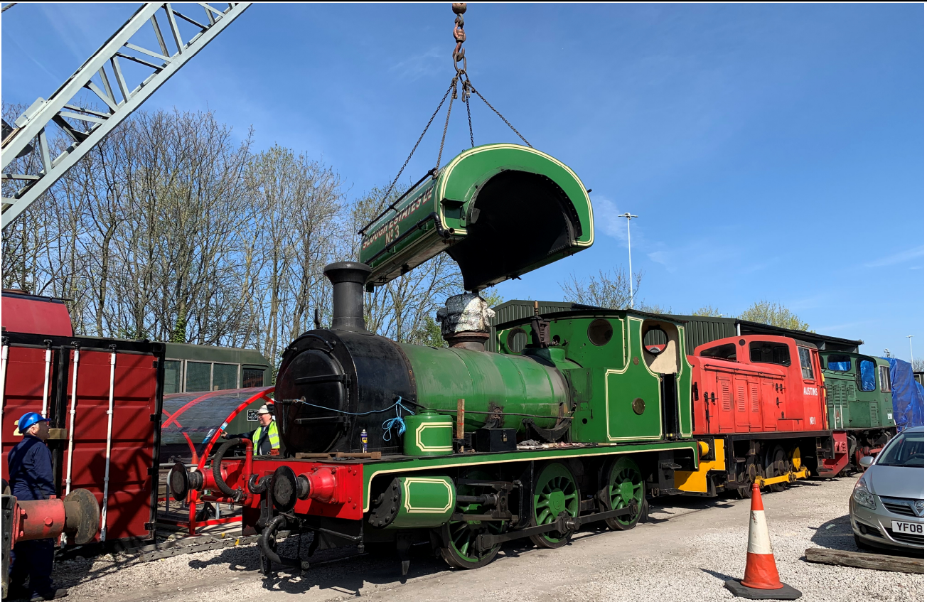
The saddle tank being lifted off SLOUGH ESTATES LTD No 3, in preparation for overhauling the boiler, 20th April 2022. © Ian Smith
