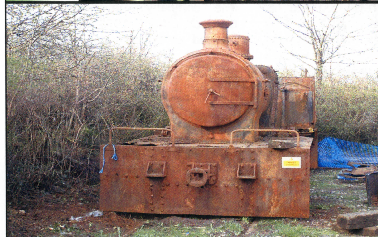
Hunslet 2-6-2T PICTON in the headshunt at Moor Road workshops, having been stripped of her side tanks and awaiting some tender loving care and attention, 4 March 2003.
