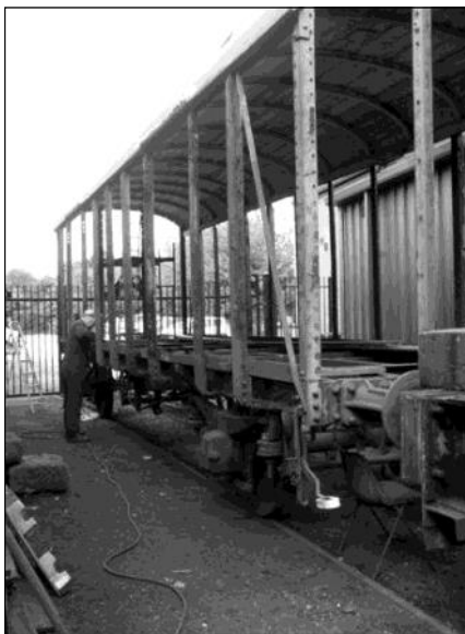
23 July 2011—Van 1074 is stripped down for conversion to a passenger carriage
