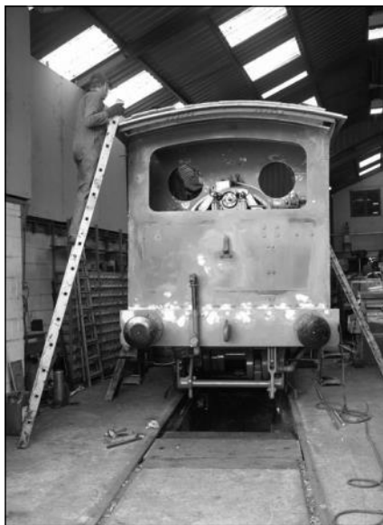
8 June 2011—1310 gets its cab roof fitted
