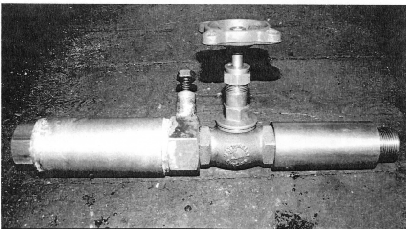
New regulator lubricator for Hudswell Clarke 0-6-OST Slough Estates No 3 (Malcom Johnson, 30 March 2012)
