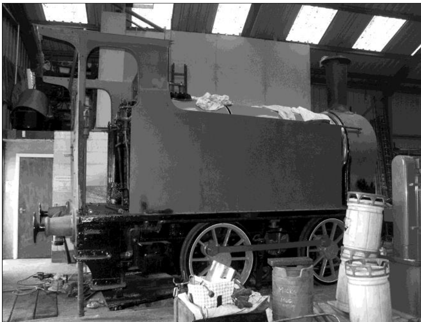
No 1310, now complete with side tanks and cab sides , looks more the part on 8 May 2011 (Andrew Johnson)
