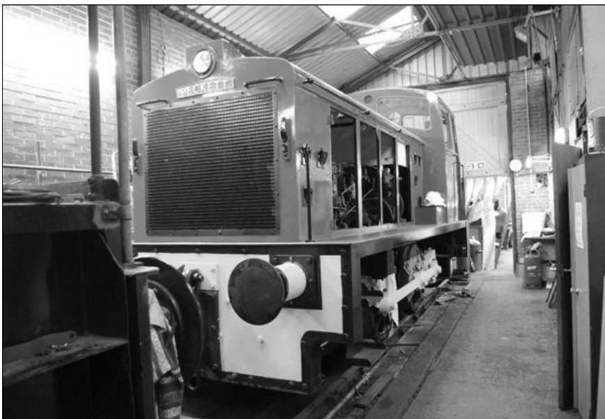
Peckett 0-4-0DM G20 class 5003 of 1961 Austin's No.1 receiving a new coat of paint in the Moor Road paint shop facility on 23 April 2011 (Ian Dobson)
