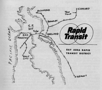
The tube, designed to withstand the most severe earthquakes, will be 130 feet below the surface.
