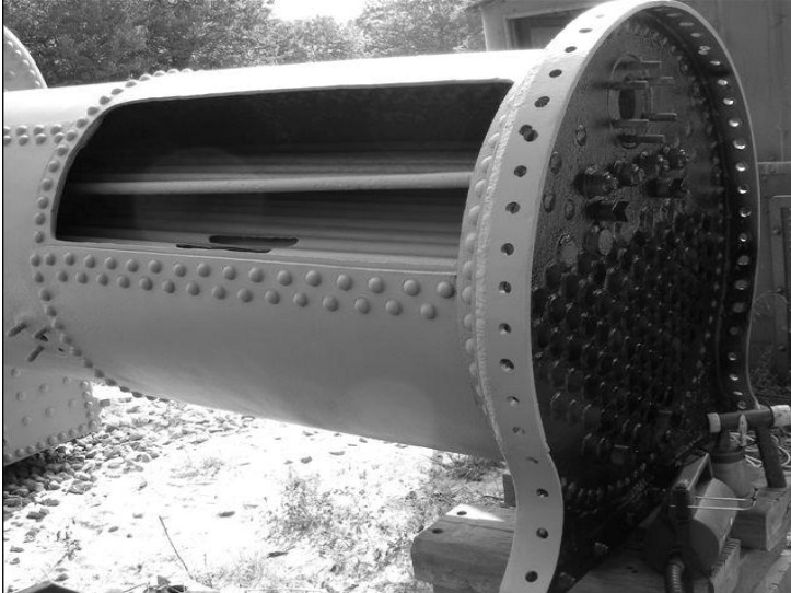
ABOVE: 19 September 2009, and Matthew Murray's old boiler has been sectioned for exhibition purposes, and is in the course of being sandblasted and painted in primer, undercoat and finished coat (Howard Bishop)
