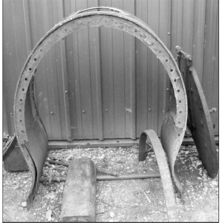
ABOVE: The smoke box from Matthew Murray , was found to be beyond repair, and has been removed from the boiler.
