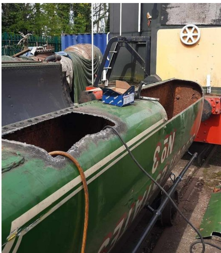
Two of the holes in the tank bottom, showing some of the riveted joints.
