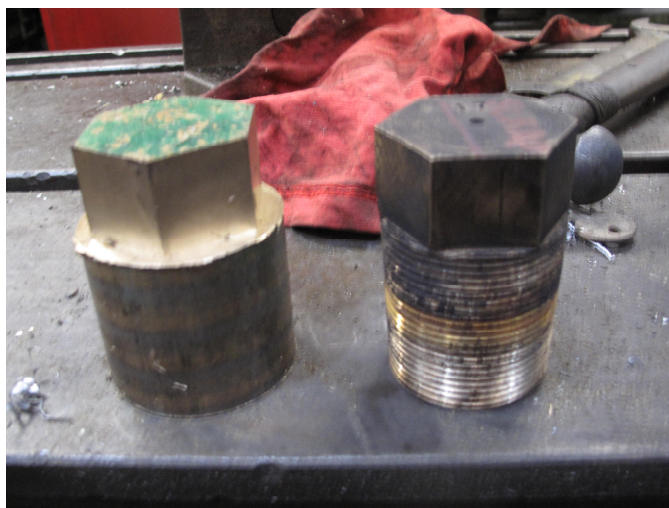
Washout plugs: on the left a new one waiting to have the screw thread cut, on the right one of the old ones.
