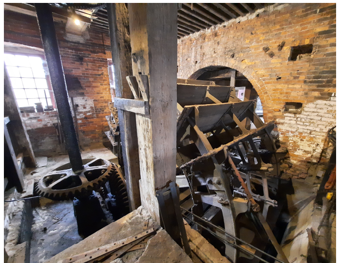
Left: The mill building seen from above the weir. Right: A waterwheel and line shafting that drove machinery across the site.
