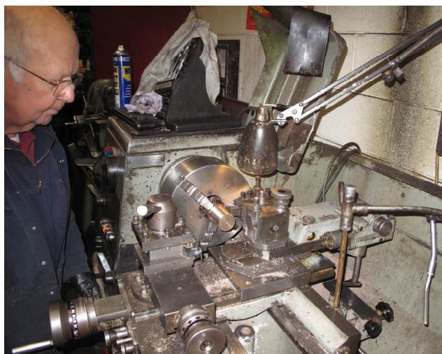
Malcolm Johnson using the lathe to cut the screw thread on one of the new washout plugs.
