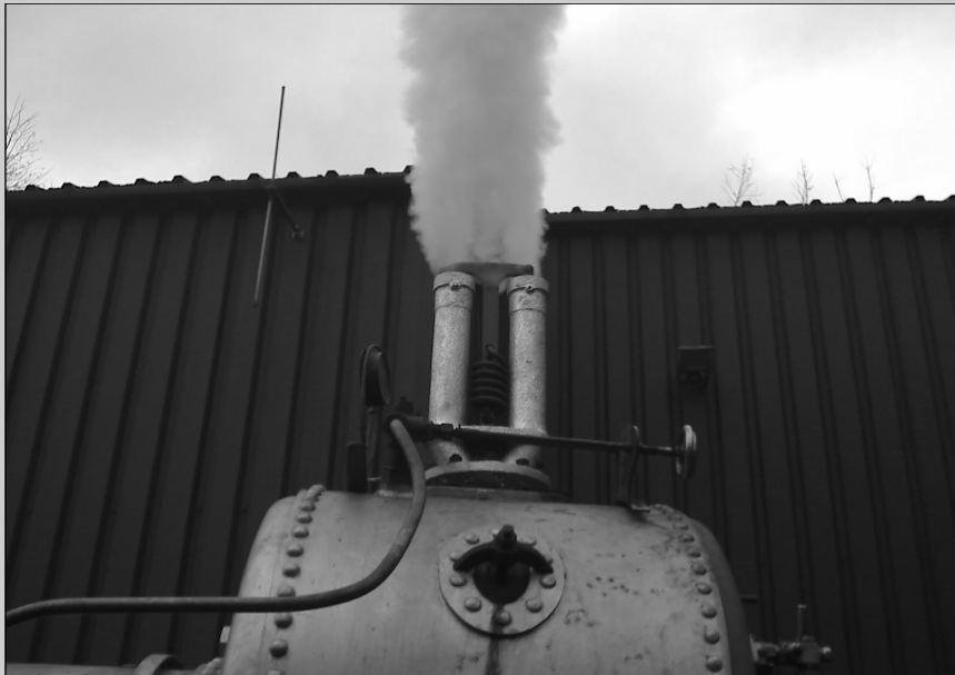
The safety valves lift on the boiler of 1601 Matthew Murray during its steam test as described in this accompanying article (Steve Roberts)
