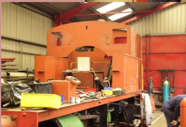
Left: New cab under construction on Hawthorne Leslie 0-4-0ST HL3860 of 1935 Percy
