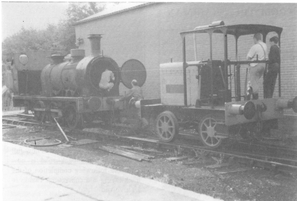
Courage , with a little help from her friends, draws the old tubes from 67's boiler, in September 1996. Photos: Graham Smith
