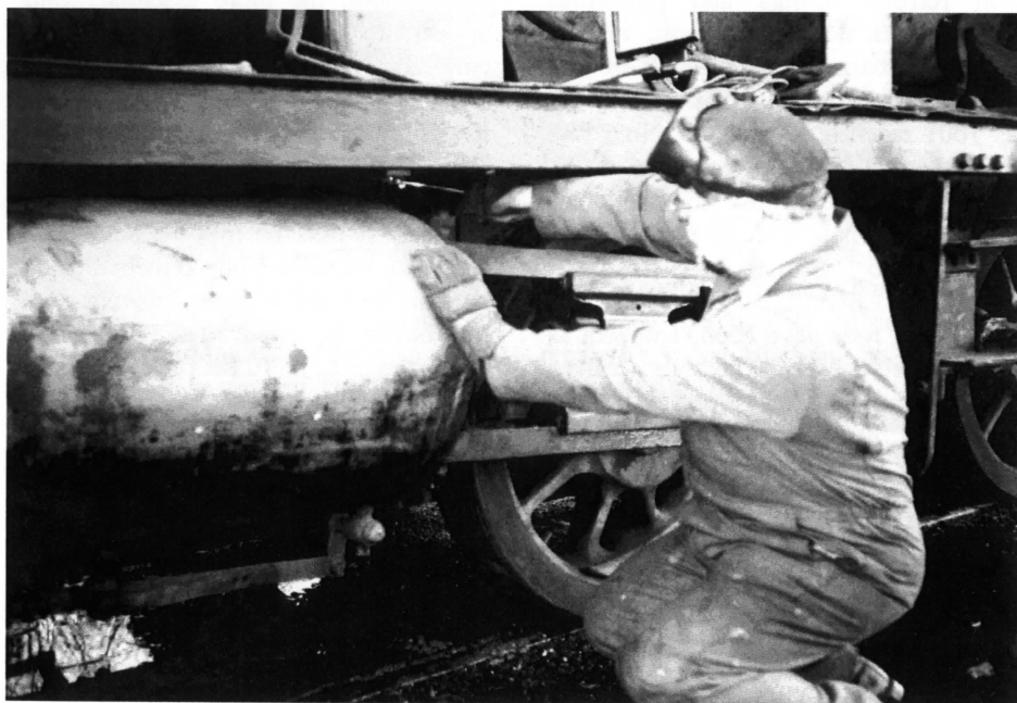
Bill Turnpenny removes a sandpipe from No.6. The sandboxes have to be removed to gain access to the bolts securing the boiler to the cylinder casting.
