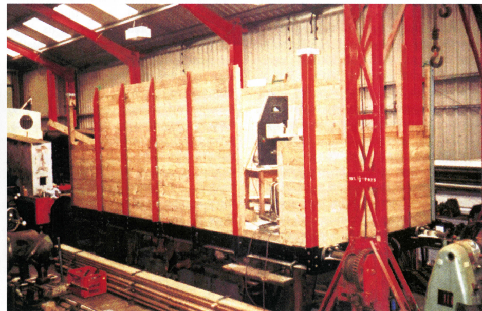
BELOW the LNER Ballast Brake van is beginning to look more like its old self as the new timber sides and ends are fitted to the framework.
