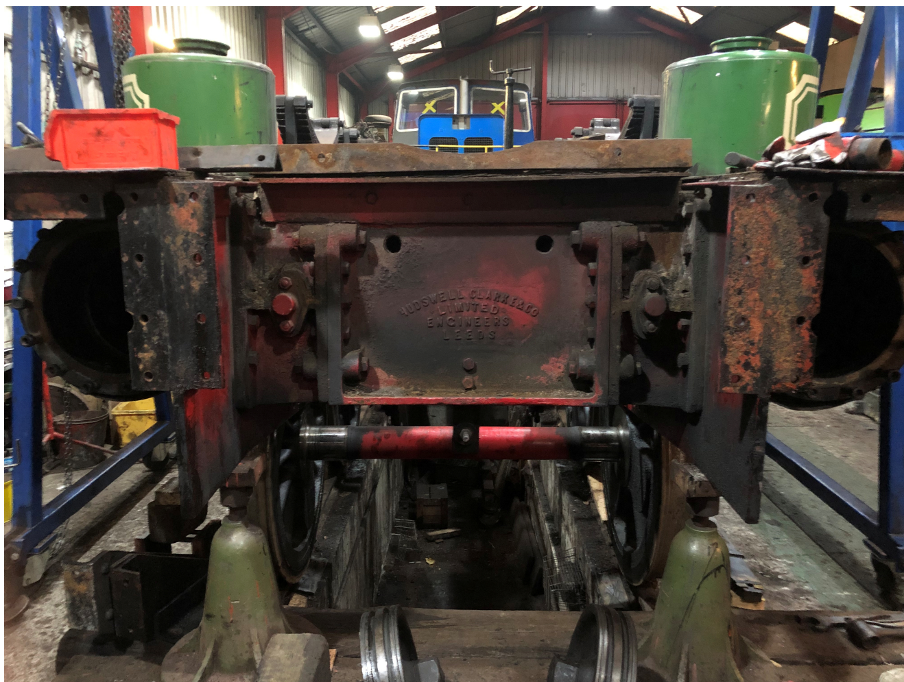
The front of HC 1544 "Slough Estates No. 3" with the bufferbeam removed, showing the cast frame stretcher which will almost certainly need to be replaced,
