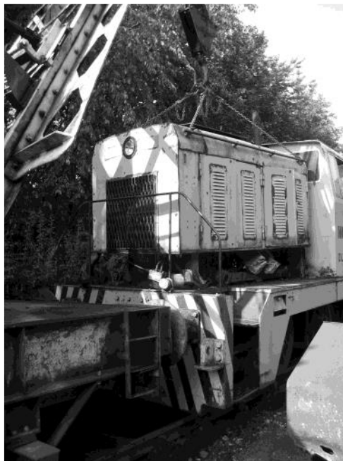
On 23 September 2006 Andrew Briddon's Hudswell Clarke 0-4-0 D1344/65 is seen having its engine cowling, removed prior to engine removal for overhaul. (Peter Briddon)
