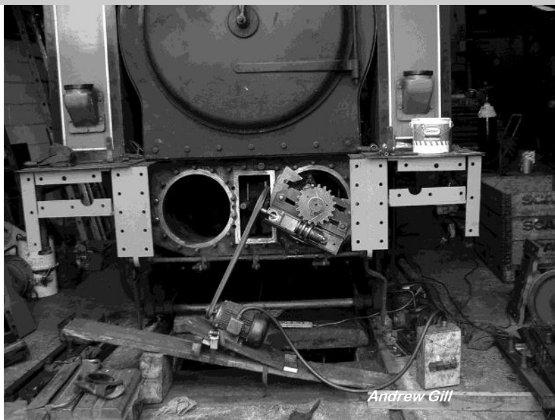
REPAIRS TO MSC 67 —The picture was taken on Sunday 15 June 2008 at the Middleton Railway engineering workshops. The picture shows a cylinder on Hudswell, Clarke 1329, (Manchester Ship Canal No. 67), being bored out ready to be fitted with a liner. The work is being carried out on site by Ian Riley (Engineering) Ltd of Bury. All the motion has had to be removed to allow access to both ends of the cylinders. Both cylinders are being machined, each taking around two days to set up and bore. The locomotive was taken out of service earlier in the year when it blew a piston ring. This (cylinder boring) machine was designed and built by the Riley family (of Riley's of Bury), three generations ago, and is still in use. It was even used on Wigan Pier!!
