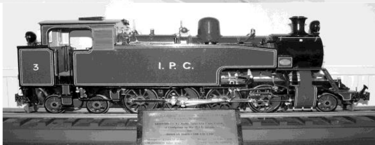
Two of the Hudswell, Clarke locos that reside at Middleton: 0-4-0ST Henry de Lacy II (HC 1309 of 1917) and fine-scale model of a 2-8-4T built in 1951 for Iraq Petroleum Company (Both photos: Howard Bishop)
