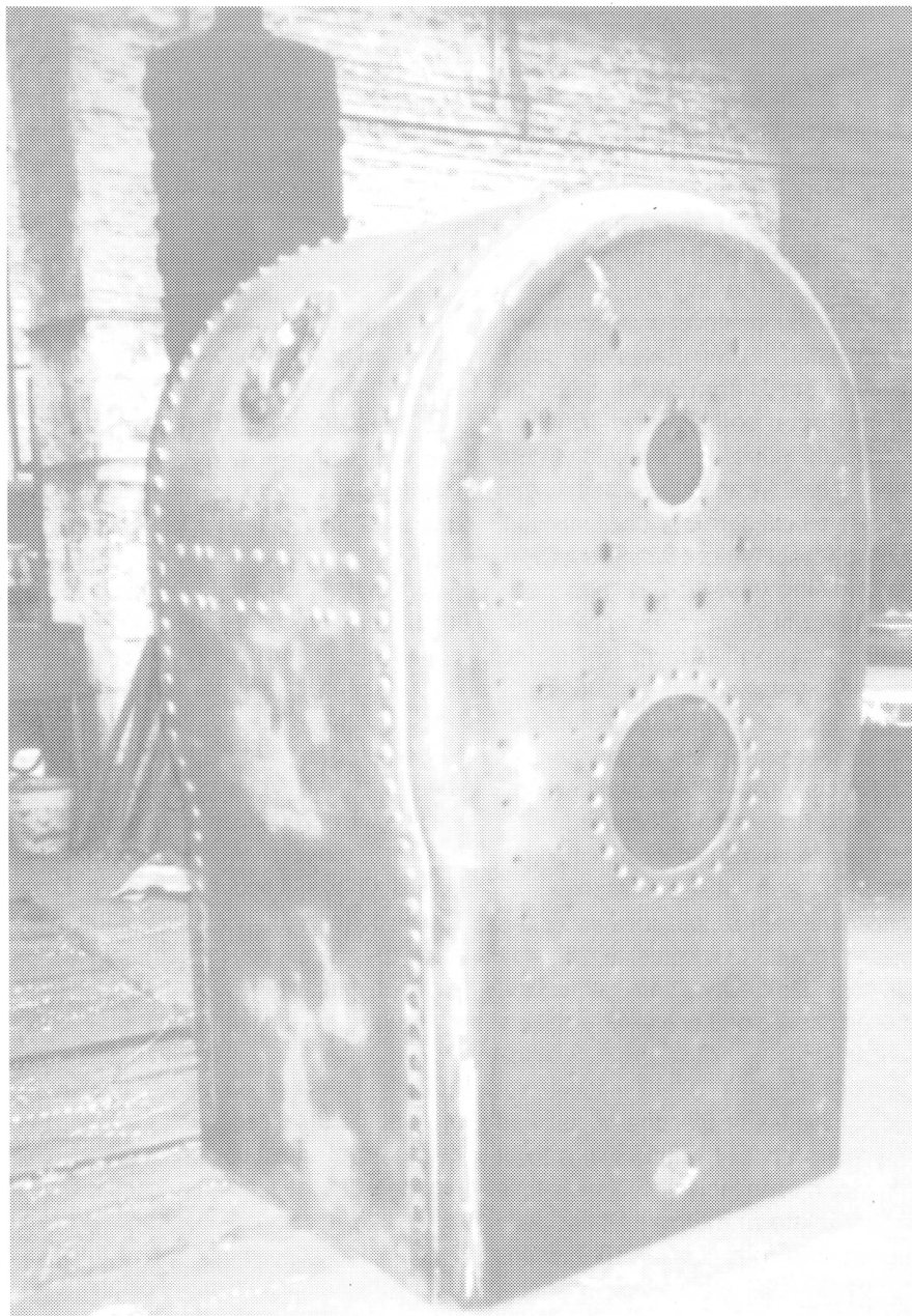
Above : New Firebox for Loco No 1601 Outerfirebox on 3rd May 2000 at Israel Newtons Works in Bradford. Photo: D Lovely
