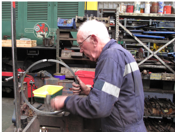
Above: Rod opening up one of the new piston rings.
