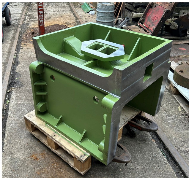
Above: the new frame stretcher, as delivered, looking at the front left-hand corner. The inverted U shape fits round the valve chest covers.
