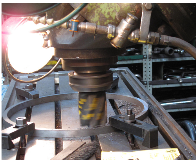
Above: one of the new piston rings being machined to size.
