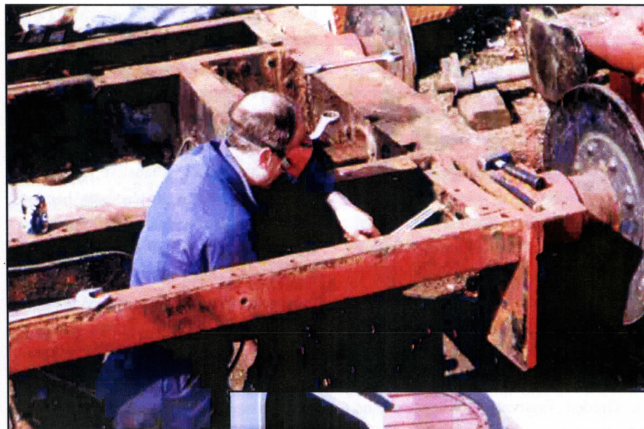
ABOVE: Graham Parkin burns off the rivets that hold the rather bent buffer beam to the frames on No.6.
