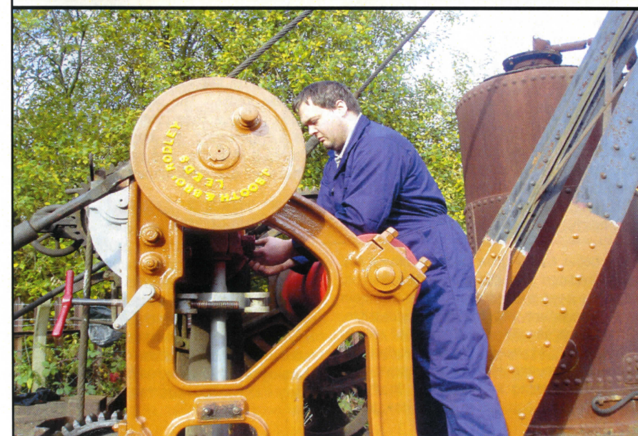
Andrew "Frankie" Parsley examines the winding gear of the 1879 built J. Booth & Bro, Rodley, Leeds, 2-ton crane, preparatory to lowering the jib to enable restoration to progress, 18 October 2003.
