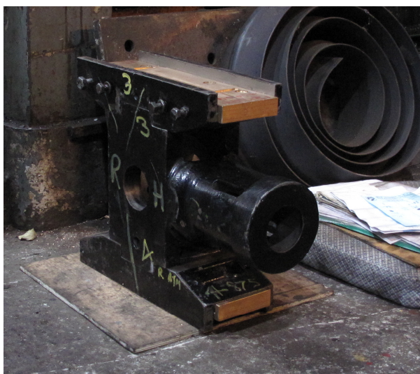
A crosshead with its new gunmetal slippers.
