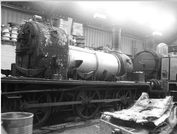
Manning Wardle 0-6-OST (1601 of 1903) Matthew Murray in the workshops stripped down for maintenance as described in this article, 23 November 2008. ( Andrew Johnson )
