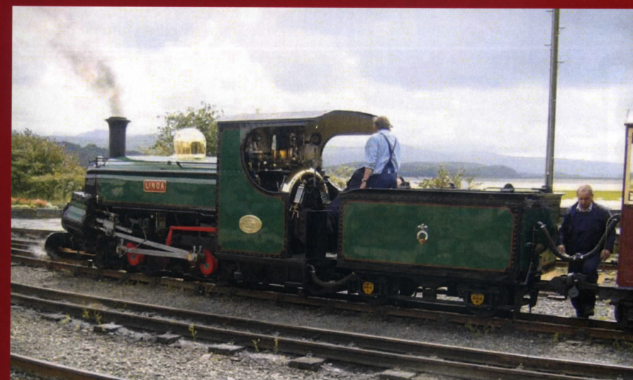
Leeds built Hunslet 0-4-0ST locomotive 580 of 1893 Linda in new green livery on 7 August 2011 at Pont Croesor on the Welsh Highland Railway (above) with the train connecting with the 1000 hours from Caernarfon (on adjacent line), and after arriving at Porthmadog on the Ffestiniog Railway via the tramway street crossing (below)
