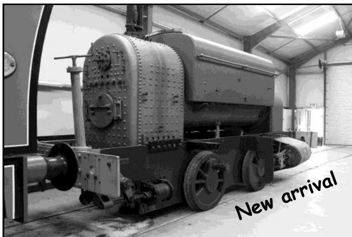
Manning Wardle 0-4-0ST No. 1795 of 1912, sits inside the Engine Shed on the day of its arrival at Middleton, 20 April 2006. This was a "special build" locomotive, after the style of their 'P' class engines, and designed for heavy duty work, having been in preservation since August 1969. For more details please see www.manning-wardle.moonfruit.com
