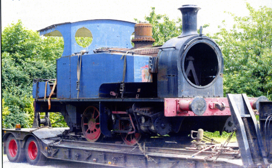
Hunslet Engine Company 14" 0-4-0T No. 1648 of 1931, and owned by the 1338 Trust, arrived at Moor Road from Ruddington on 16 June 2004. The locomotive joins the Leeds Locomotive Collection for eventual restoration. It last steamed in the late 1960s. (HWB)
