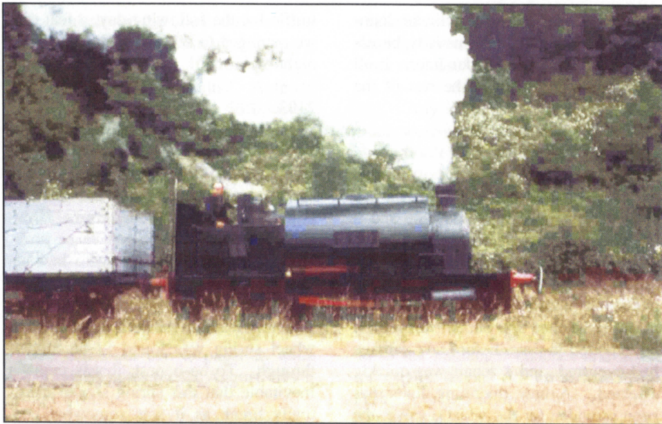
ABOVE Currently under overhaul in our workshops is Hunslet 0-4-0ST No.11 (works No.1493/25). It is seen here after initial preservation and whilst in use on the Battlefield line. It was originally provided with a low, roofless cab to enable it to negotiate a low bridge. The intention is to provide a more orthodox cab. (Photo by Barry Williamson)
