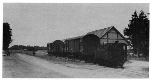
The interchange point between the gauges on the Hummlinger. To the left a standard gauge diesel is undergoing acceptance trials, while in the foreground Werlte 1 e a v e s with a train of standard gauge wagons on narrow gauge transporters.
