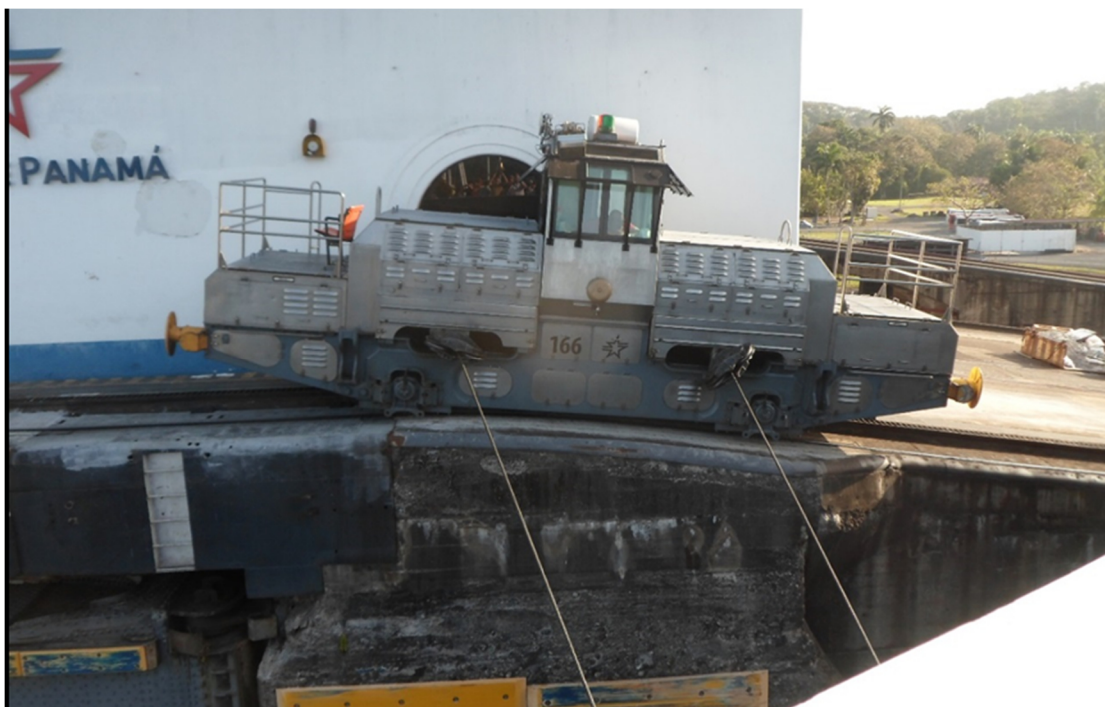
A rack and pinion locomotive showing the guide wires.
